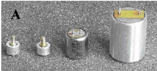
Figure 1. Two examples of the test version of the GSS sensor in comparison with Geo Space's Commercial Geophones GS-14-L3 (in the middle) and GS-20DX (on the right)
