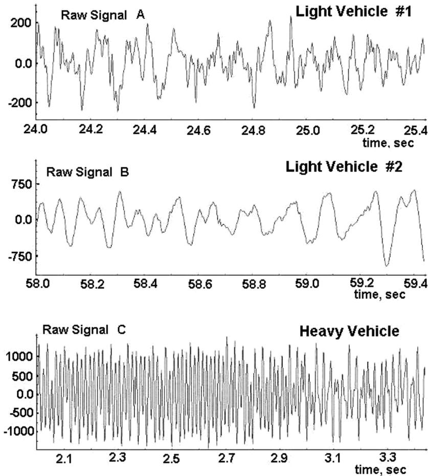
Figure 8. Examples of the raw signals for light and heavy vehicles.
