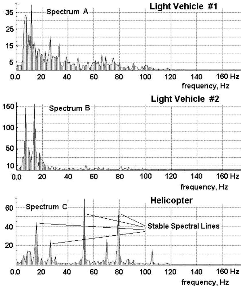
Figure 9. Signal spectra for various targets (A, B – light vehicles, C – helicopter).
