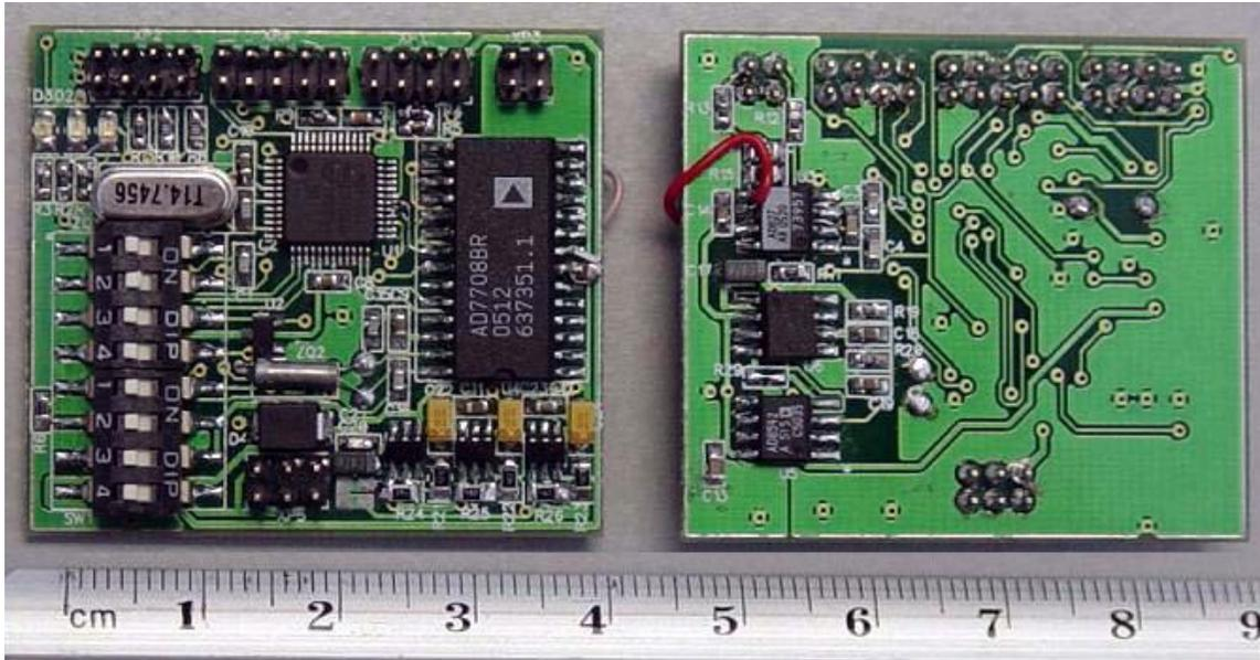
Figure 1. The GSS seismic detection module board.
