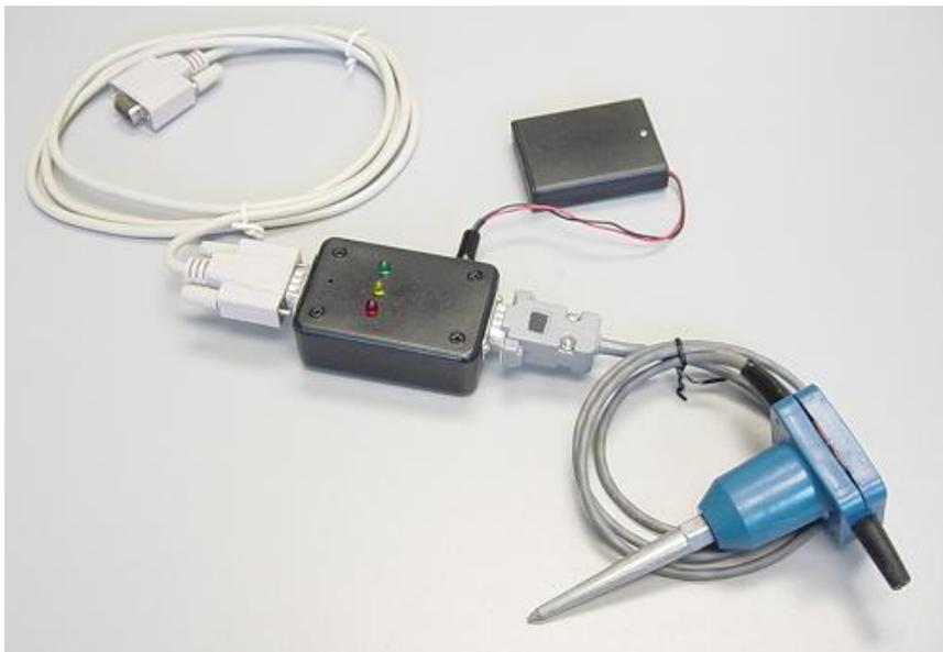
Figure 3. Field testing hardware comprising geophone, processing box, battery, and a PC interface cable.
