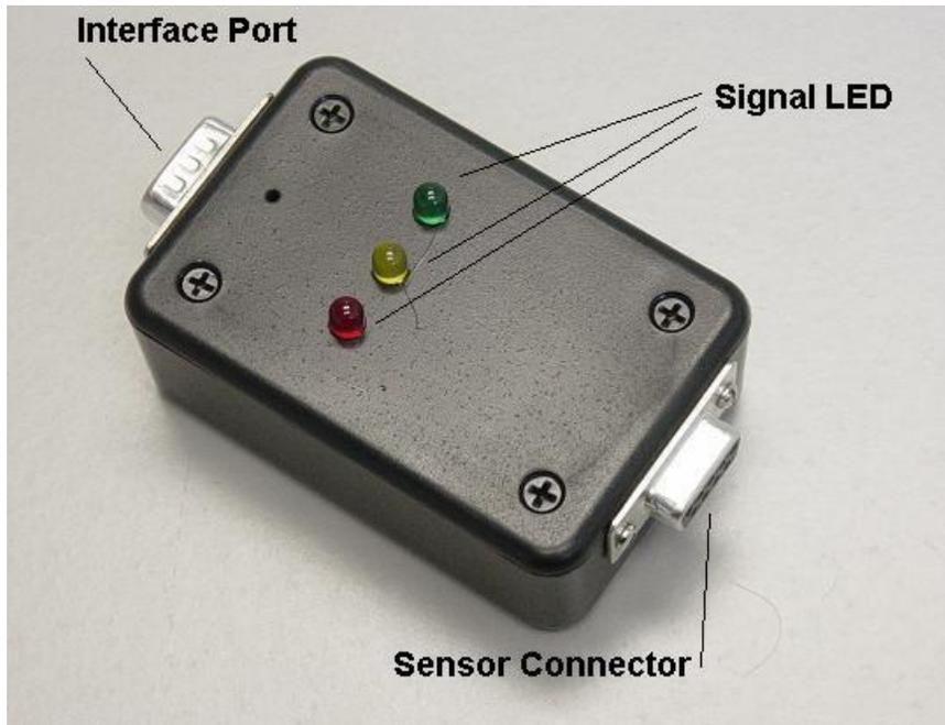
Figure 2. Detection hardware box with signal LEDs, a sensor connector and an interface port.
