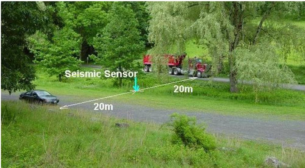
Figure 6. Layout of the seismic sensor relative to traffic in the second testing area.
