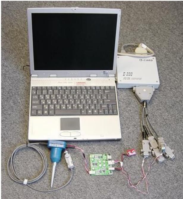
Figure 2. Seismic system components used in the field test.
