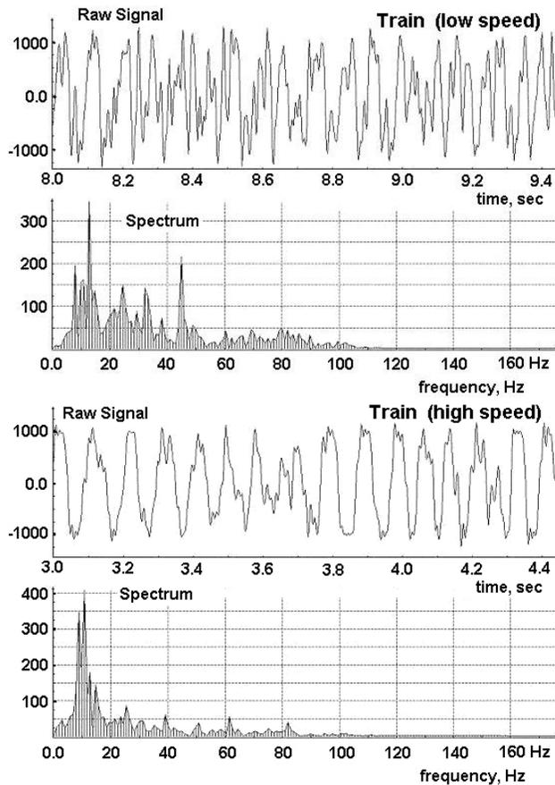
Figure 5. Raw signal and its spectrum for low and high speed train.
