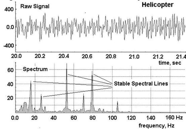
Figure 7. Raw signal and its spectrum for a helicopter.
