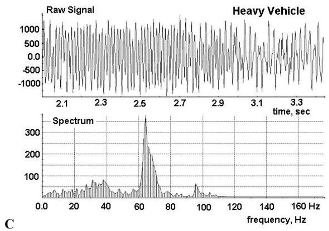
Figure 6. Raw signal and its spectrum for light (A, B) and heavy (C) vehicle. The records represent moments when the distance between the seismic sensor and the vehicles was about 5-15m. The speed of all vehicles was low (about 15-20km per hour). Figure 6A shows the signal from a vehicle that was moving in high gear with constant speed. Figure 6B and Figure 6C show the signals from vehicles that were moving in low gear with acceleration.
