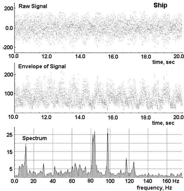
Figure 8. Raw seismic signal and its envelope and spectrum for ship.
