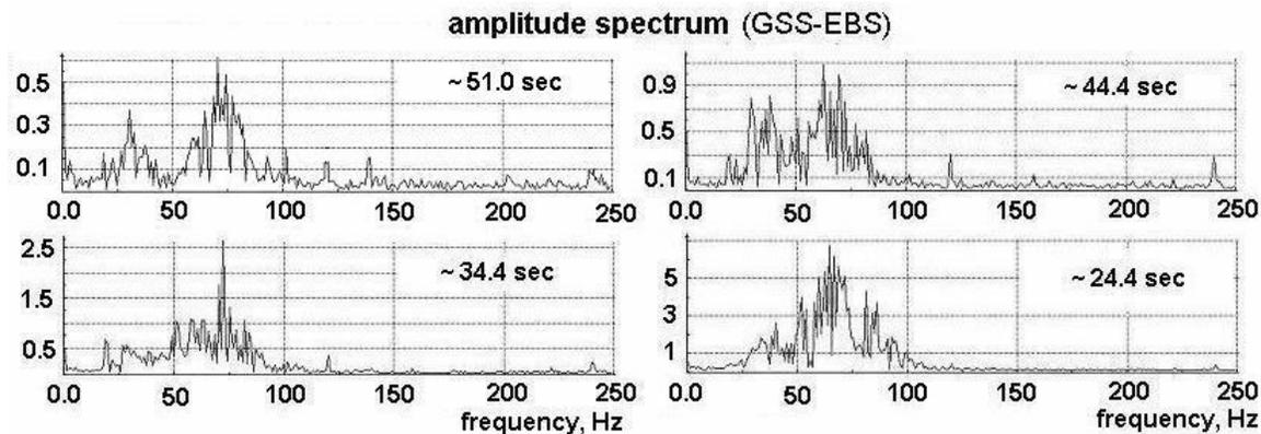
Figure 14. Amplitude spectrum of the footstep signals for different time marks (GSS-EBS).
