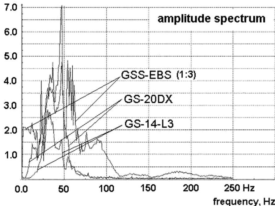
Figure 5. The amplitude spectrum of the seismic signals recorded by the GSS-EBS, GS-14-L3 and GS-20DX geophones and shown in Figure 4.
