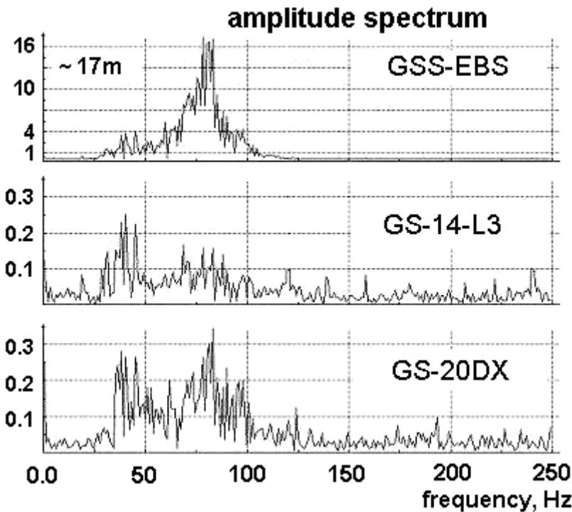
Figure 13. The amplitude spectrum of the seismic signals shown in Figure 12.
