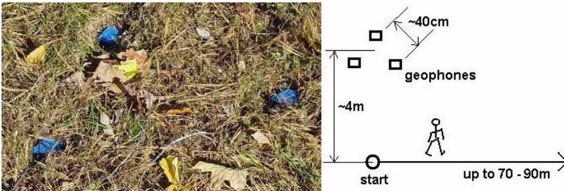
Figure 9. Test layout of geophones used to collect footstep data in both areas.
