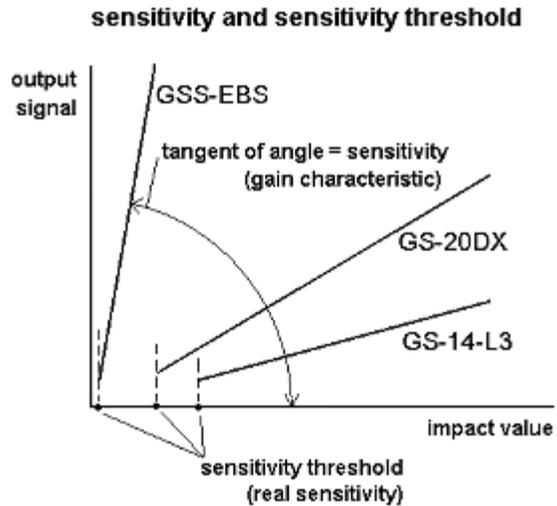
Figure 16. Higher sensitivity and lower sensitivity threshold of the GSS-EBS in comparison with commercial geophones.
