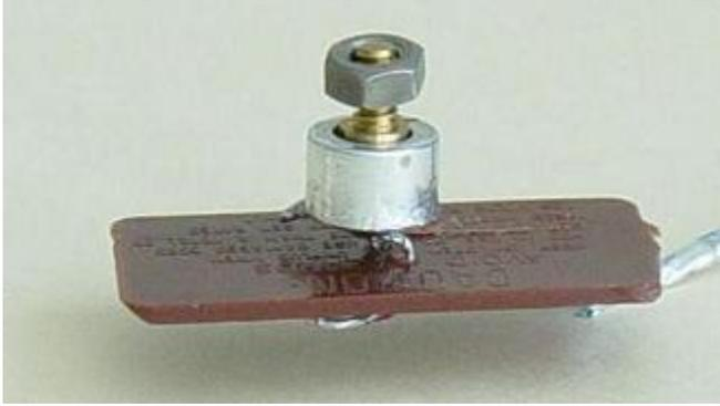
Figure 1. GSS sensor with middle replaceable mass on a board for secure attachment to a vibration stand (lab test) or to a land case of a standard geophone (field test).
