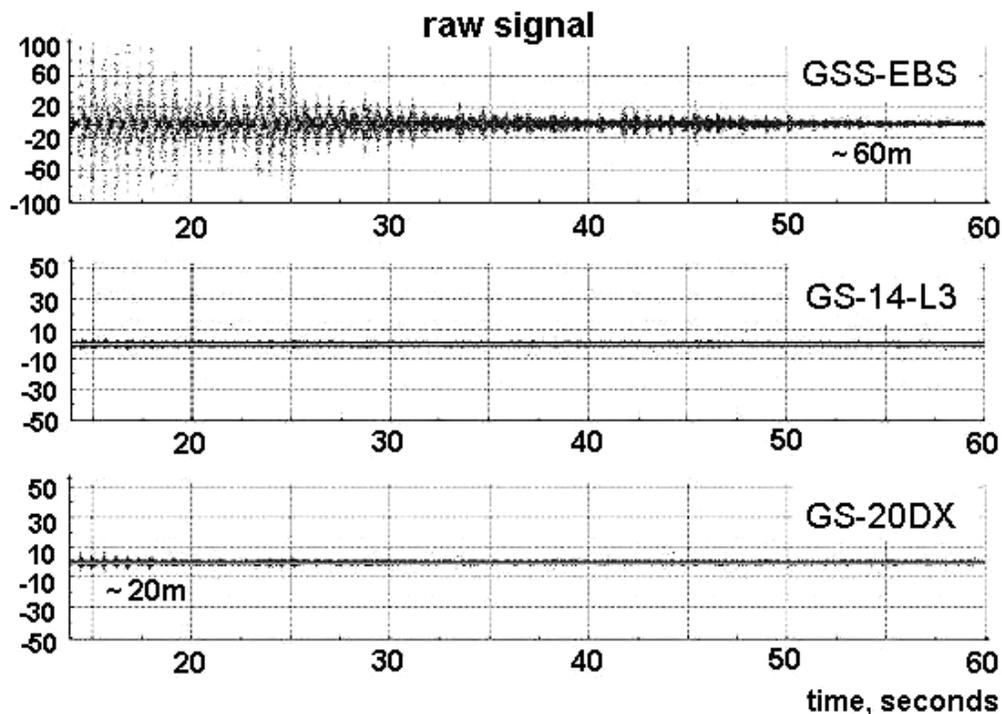
Figure 10. Recordings of the same seismic footstep signal (area #1). Last 45 seconds are shown.
