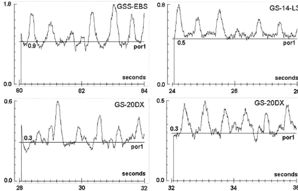
Figure 15. Envelopes of the same seismic footstep signal recordings with the time frames corresponding to the maximum of the footstep detection range. The level “por1” shows the value of the raw signal root-mean-square.
