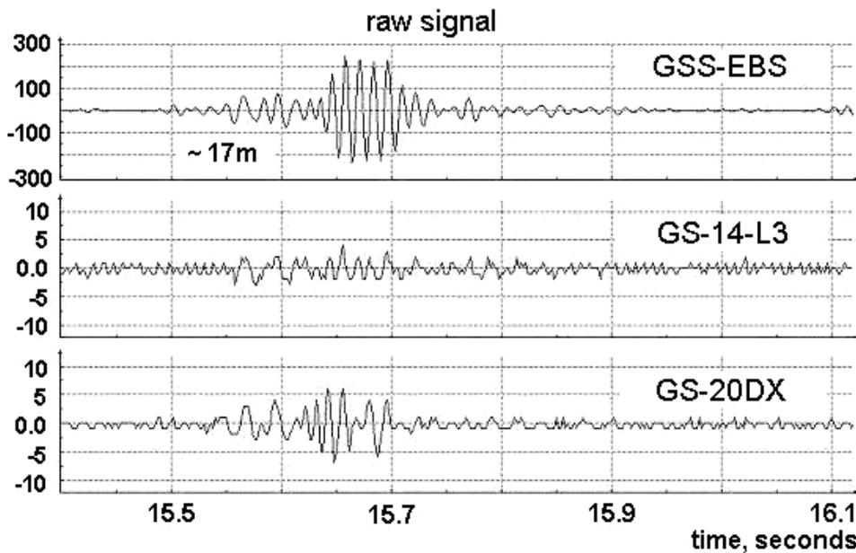
Figure 12. Highlight from Figure 10 of an area with a one step signal (Distance is about 17 m).
