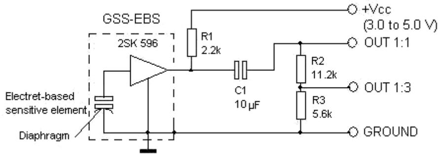
Figure 3. Sensor powering circuit.
