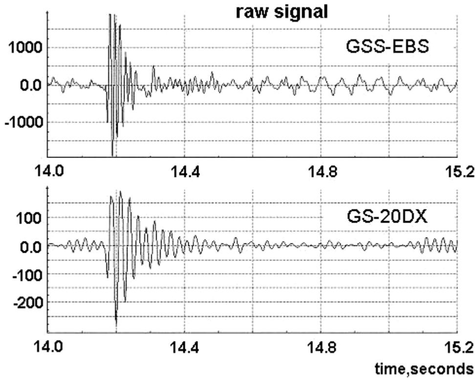
Figure 6. Records of the same seismic signal by the GSS-EBS and GS-20DX geophone. Weak impact and use of the amplifiers with gain of about 10,000 for all geophones.
