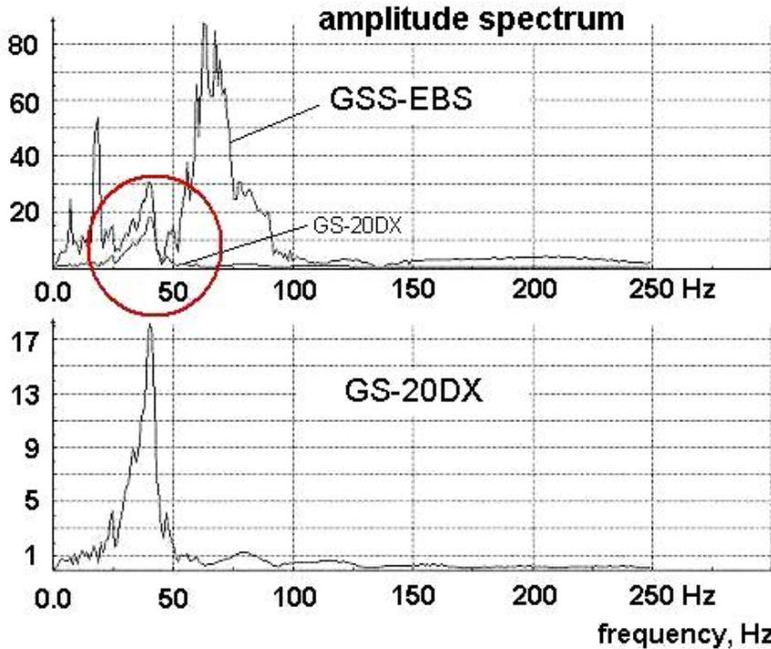
Figure 7. The amplitude spectrum of the seismic signals recorded by the GSS-EBS and GS-20DX geophone and shown in Figure 6.
