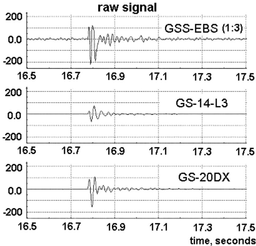
Figure 4. Records of the same seismic signal by the GSS-EBS and two different geophones GS-14-L3 and GS-20DX. Strong impact and using of an attenuator (1:3) for GSS-EBS.
