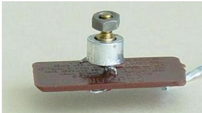
Figure 2. GSS sensor on a board for securely attaching to a vibration stand (lab test) or to a land case of a standard geophone (field test).
