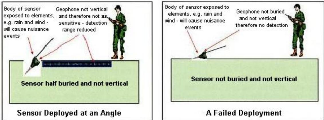
Figure 1. Issues of the angular deployment of seismic sensor.
