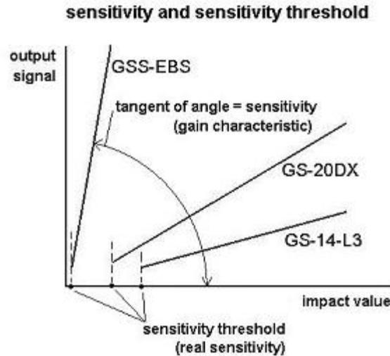
Figure 9. Higher sensitivity and lower sensitivity threshold of the GSS electret based sensor in comparison with commercial geophones.
