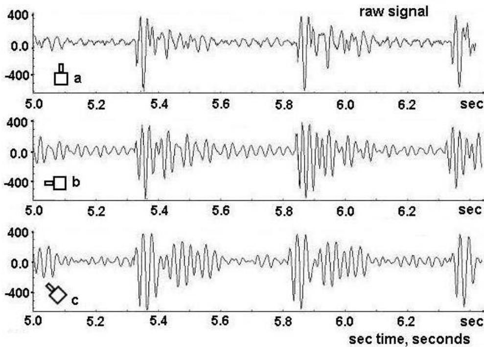
Figure 4. Records of the same seismic signal by the different sensor orientation as shown in Figure 3.
