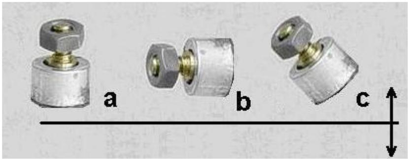
Figure 3. GSS's sensor testing by its different orientation on a vibration stand.
