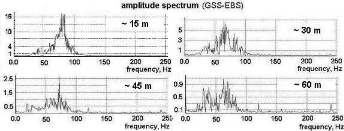
Figure 6. The amplitude spectrum of the footstep signals for different distances between a walking person and seismic sensor.
