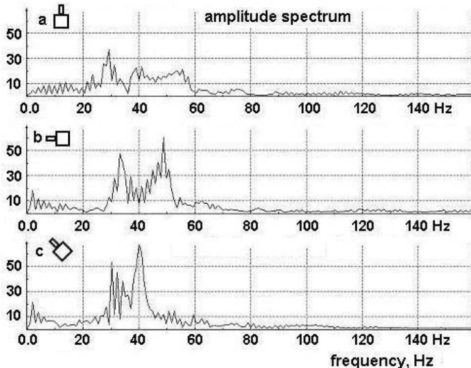
Figure 5. The amplitude spectrum of the seismic signals recorded by the GSS sensor and shown in Figure 4.
